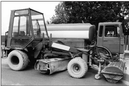
Equipment used to expose the surface aggregate.
